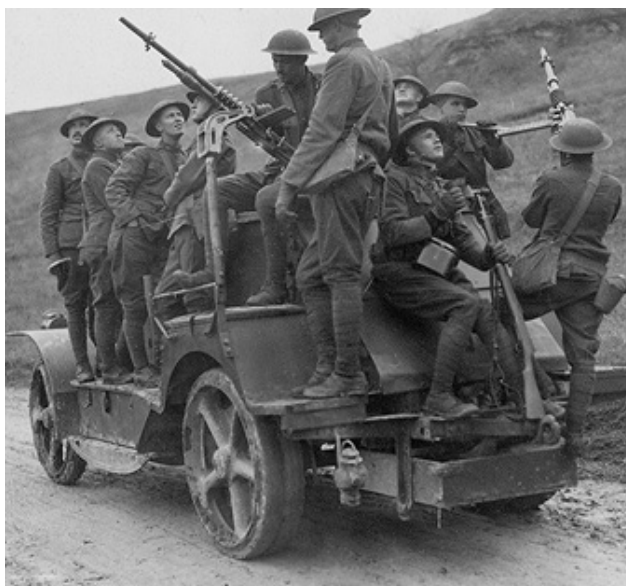
Tender of an Observation Balloon Mounted with Two Machine Guns for Anti-Aircraft Defense
