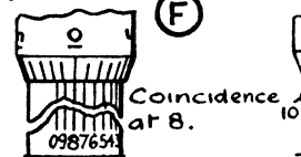
Fig. 172.—Sample Settings of Micrometer Caliper, reading to \frac{1}{1000} inch.
