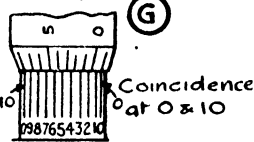
Fig. 172.—Sample Settings of Micrometer Caliper, reading to \frac{1}{1000} inch.
