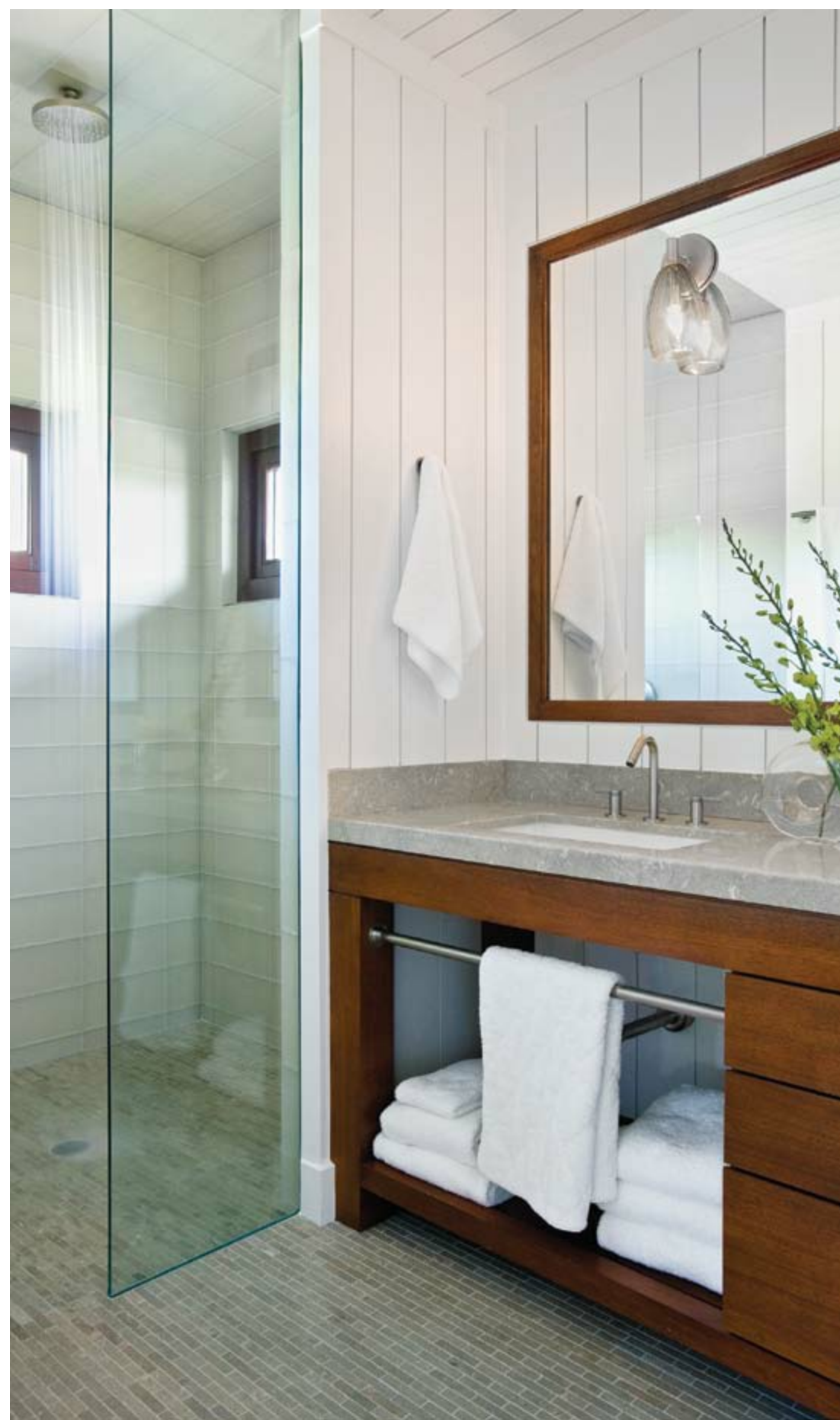
above • The simple glass splash guard helps to keep water in check in this curbless shower, particularly
